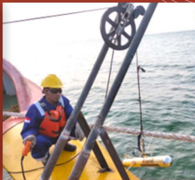
SIDE SCAN SONAR MODEL EDGETECH 4125 INSTALLATION
