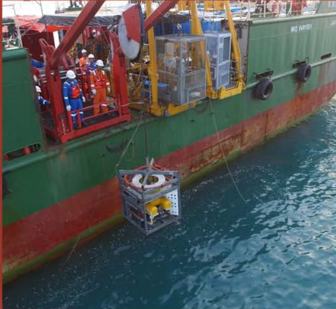
ROV SEMI WORK CLASS SEA EYE PANTHER 946 DEPLOYMENT FOR UNDER WATER PLATFORM INSPECTION (UWPI)
