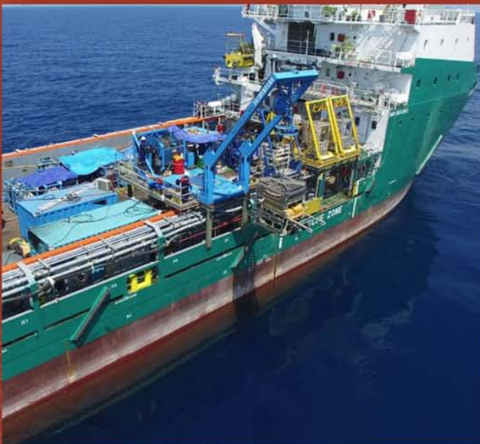
ROV SEMI WORK CLASS SEA EYE PANTHER 946 DEPLOYMENT FOR PIPELINE INSPECTION
